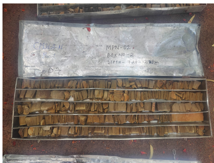
Photo-14.3: Photograph of half splitted borehole cores of MPN-02
