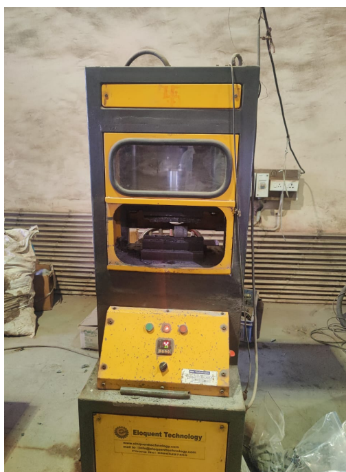
Photo-14.2: Photograph showing core splitter used to split borehole cores
