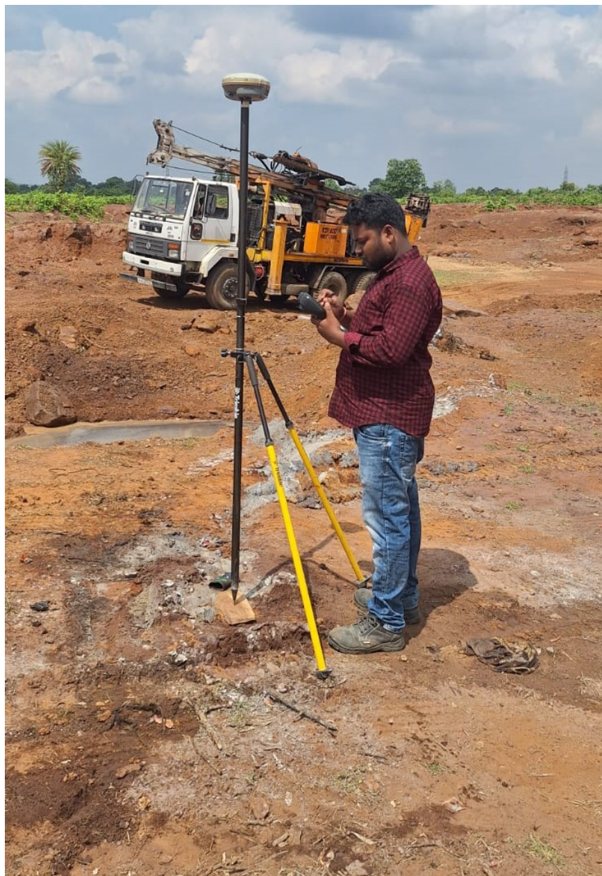
Photo-11.1: DGPS (Make-Trimble GNSS System, Model-R8s)
